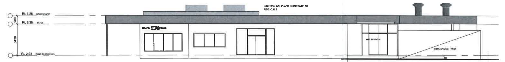
■ WEST SELECT APPLIED FINISHES, RENDER & PAINT ALL BRICKWORK, NEW ALUMINIUM FRAMED DOORS
